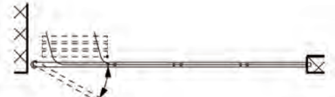
Straight installation with parallel stacking and pivot door.
