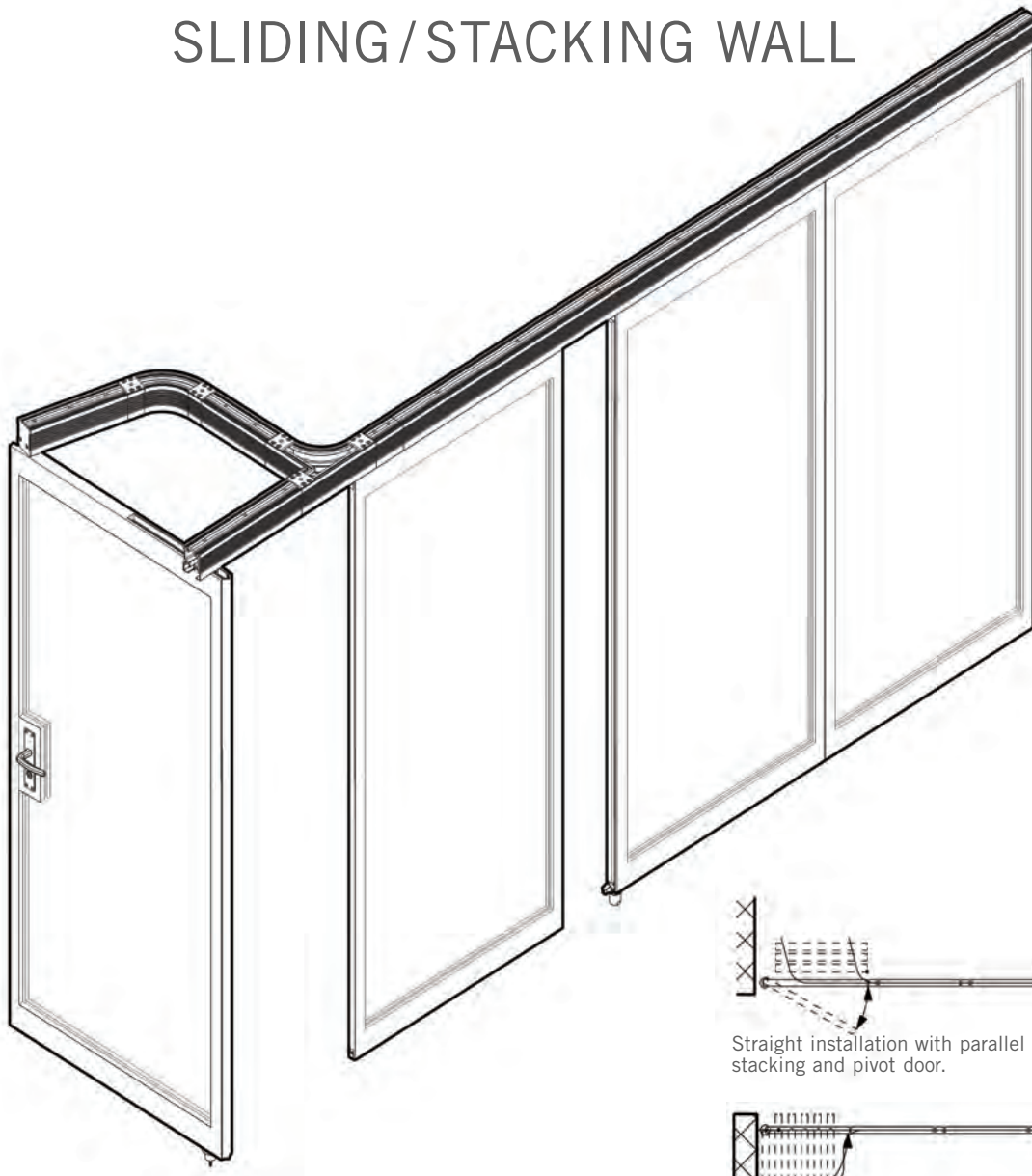
Installation with a 90° change in direction stacking and pivot door.
